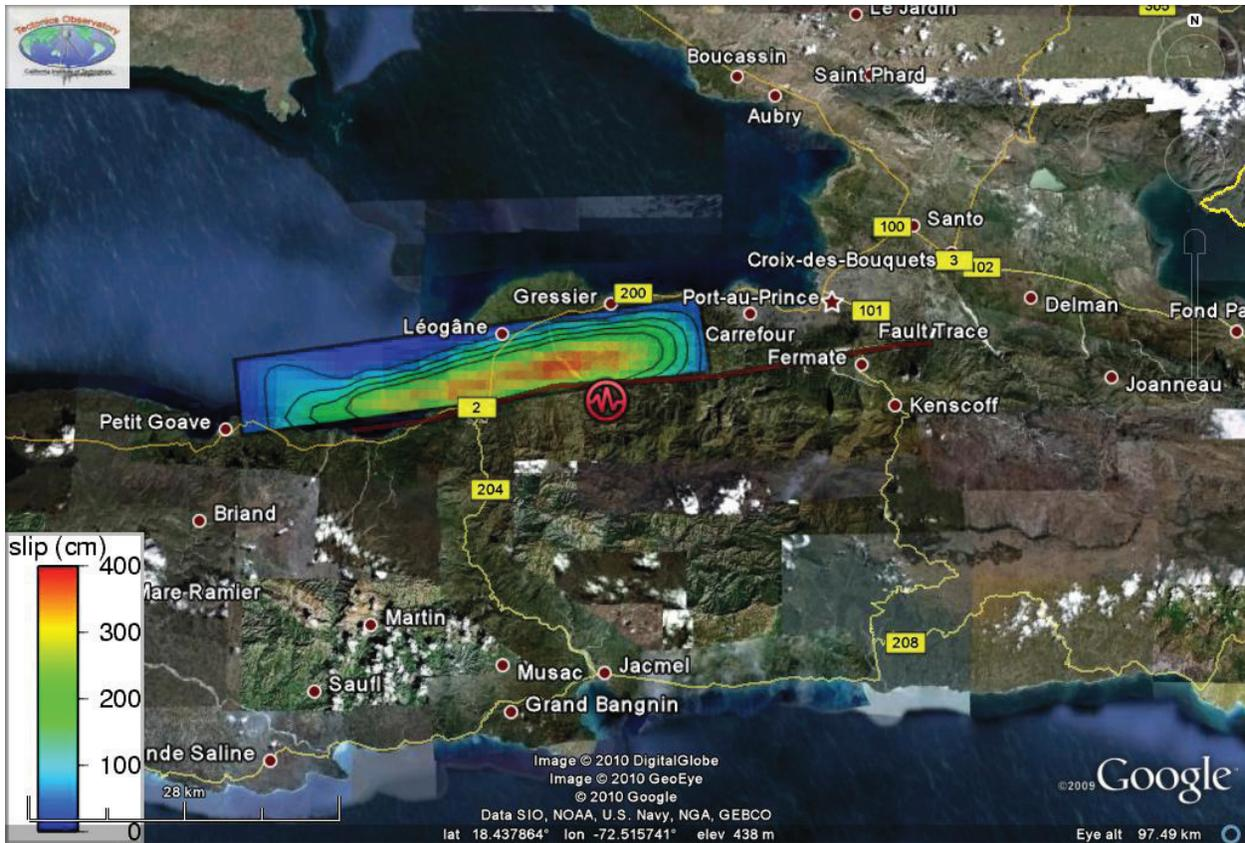
**Figure 5.1** Estimated fault rupture distribution for the 2010 Haiti earthquake ([http://tectonics.caltech.edu/slip\\_history/2010\\_haiti/](http://tectonics.caltech.edu/slip_history/2010_haiti/)) and location of major city centers.
