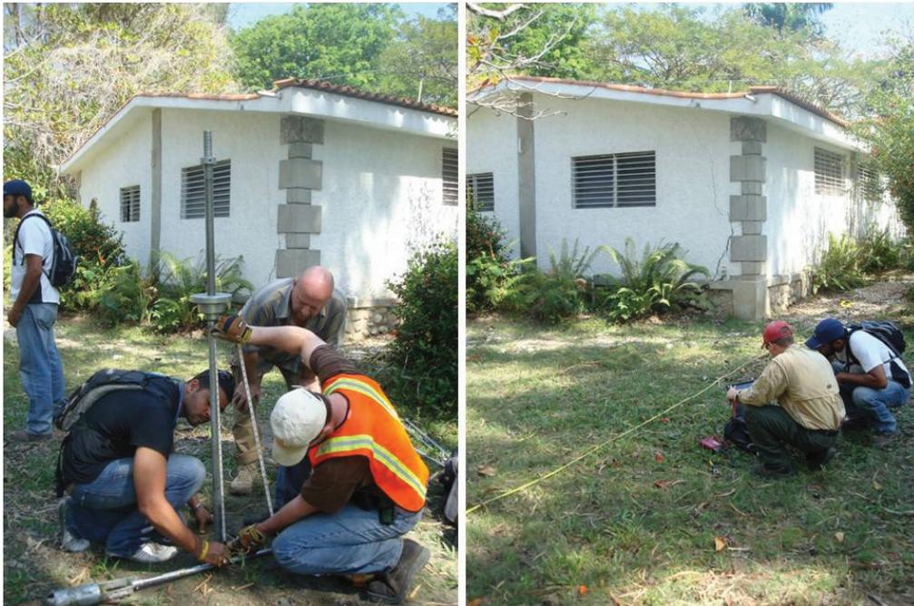
**Figure 7.14.** DCPT and SASW testing performed at coastal failure site near village of Fouche. Approximate image coordinates: 18°25'35.12"N, 72°43'31.61"W.
