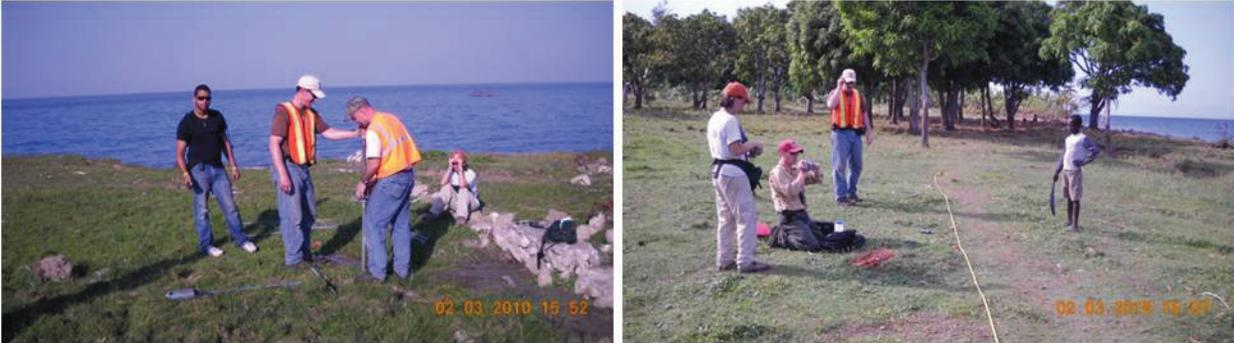
**Figure 7.22.** DCPT and SASW testing at coastal failure site near village of Grand Goâve. ( $18^{\circ}25'53.64''\text{N}$ ,  $72^{\circ}45'37.76''\text{W}$  for left image,  $18^{\circ}25'54.16''\text{N}$ ,  $72^{\circ}45'37.85''\text{W}$  for right image)
